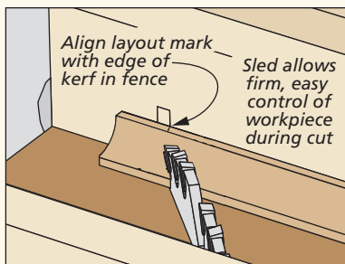
▲ Align your layout mark with the edge of the kerf in the sled and then make the cut.
